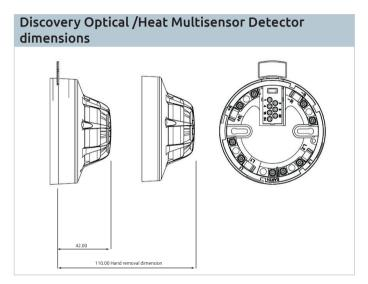
*Note:* Should be used with Deckhead Mounting Box - Part No. 45681-217 if ingress protection is required.
